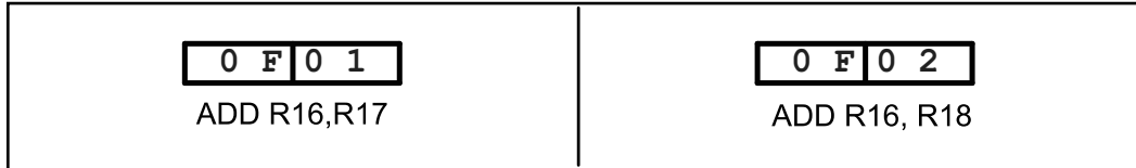
Figure 17. The Machine Code for Instruction “ADD Rd,Rr” in Hex
