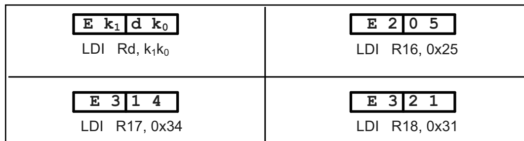
Figure 15. The Machine Code for Instruction “LDI Rd, k” in Hex
