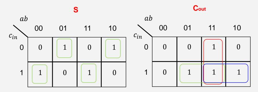
$$c_{out} = ab + c_{in}b + c_{in}a$$
