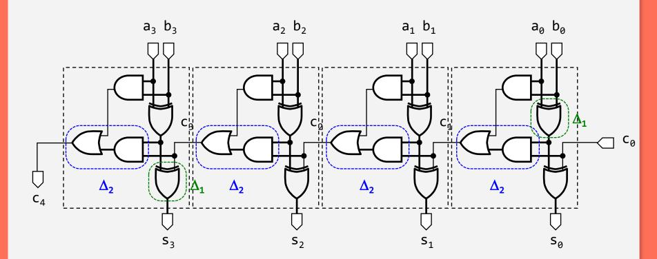
Suppose the XOR delay is  $\Delta_1$  and AND-OR delay is  $\Delta_2$ For an *N*-bit ripple-carry adder, if all inputs are present at once:
