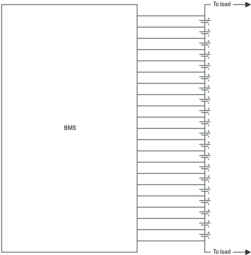
Figure 5.1 Monolithic battery management system.
