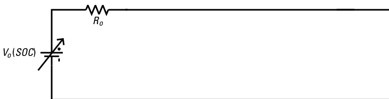
Figure 11.3 Battery representation with variable voltage source.
