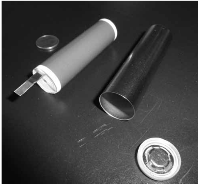
Figure 2.3 Disassembled 18650 cell showing pressure vent, enclosure, and jelly roll.
