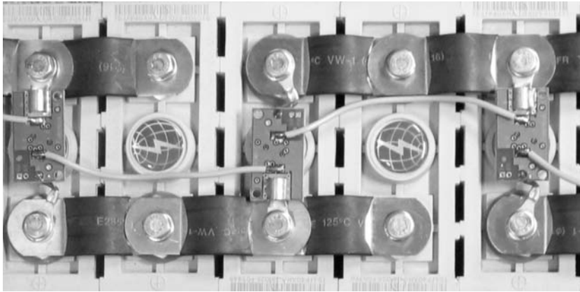
Figure 6.16 The loop antenna area: wide loop area (left—bad) and small loop area (right—good).
