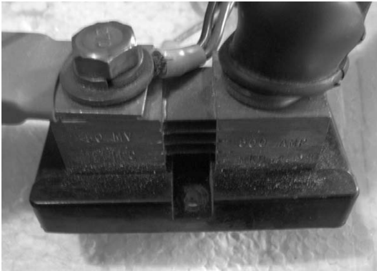
Figure 6.12 Connections to a shunt current sensor.
