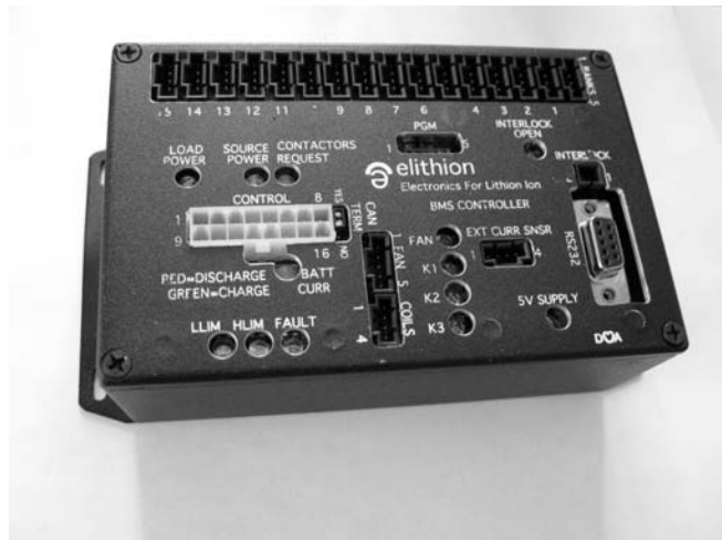
Figure 4.8 Elithion's Lithiumate, a distributed balancer.
