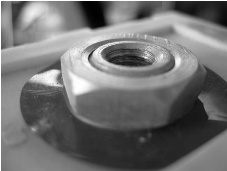
Figure 6.10 Prismatic cell terminal. A center stud is secured with a large nut. The nut must not extend past the stud. The aluminum stud must be treated with deoxidant if it is to be used with copper connections.
