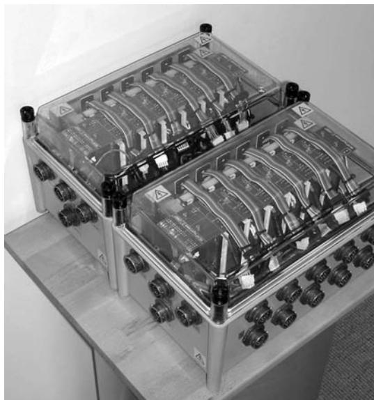
Figure 4.11 REAP's BMS for 168 cells. (Source: Stephanie Pielot, REAP Systems, 2010. Reprinted with permission.)
