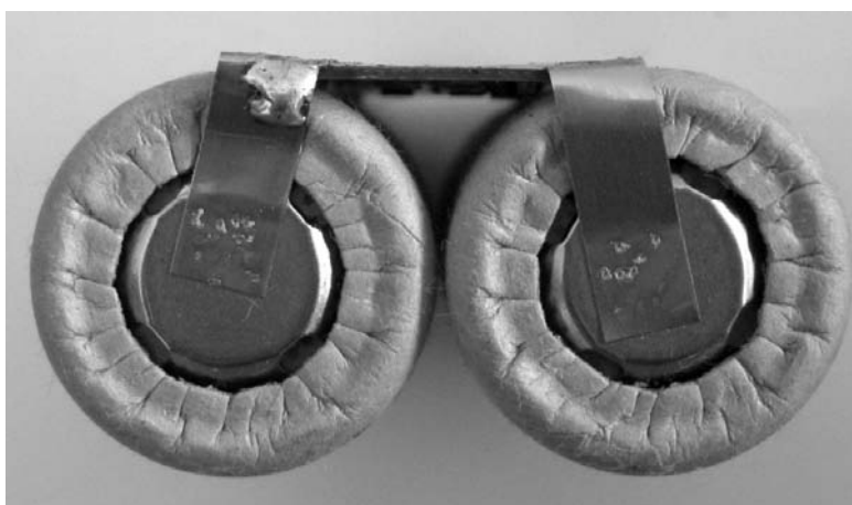
Figure 5.87 Cell board components nestled in the space between adjacent small cylindrical cells.
