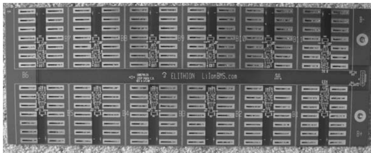
Figure 5.94 Cell board for multiple pouch cells (12S7P arrangement).
