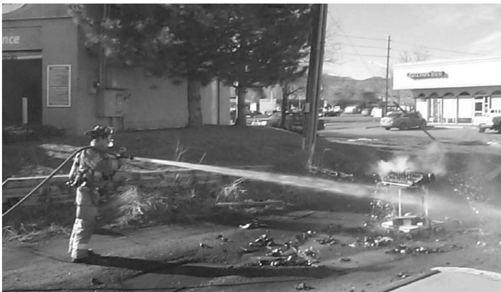
Figure 1.3 Putting out a Li-Ion battery on fire after a direct short circuit across it.
